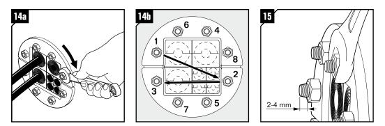
Tighten the nuts crosswise. The seal is compressed when excessive lubricant is visible between the module halves as well as 2-4 mm of the thread.
