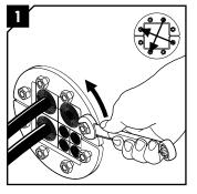
Untighten the nuts crosswise. Make sure the nuts are completely loose.
