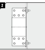
Use the flange as template for the drilling of the bolt holes.
