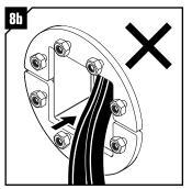
Pull the pipes/cables through. Cables shall go straight through the seal.
