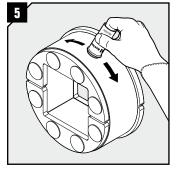
Lubricate the frame sparsely on the outside with Roxtec Lubricant if needed.
