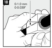
Adapt modules to cables/pipes by peeling off layers. Achieve a 0-1.0 mm gap between the two halves when held against the cable/pipe. The halves may not differ by more than one layer. The last layer cannot be removed.
