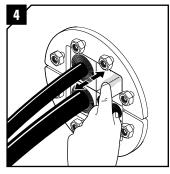
Lubricate the inside surfaces all around with Roxtec Lubricant, especially into the corners. Continue the reinstallation on page 3, step 8.
