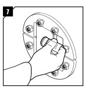
Lubricate the inside of the frame thoroughly, especially into the corners.
