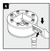
If pipes/cables are pre-routed, the frame can be cut open with a sharp lubricated tool. Note: The cut must be smooth without removing material.
