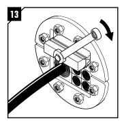
Use Roxtec pre-compression tool to make room for the final module row.
