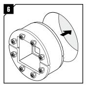
Insert the frame into the sleeve/ hole.
