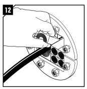
Insert the modules and cables/ pipes according to your installation plan (transit plan). Begin with the smallest modules.
