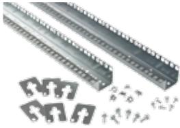
23-in. Rack Angles are available for telecom applications. They fit directly into 700-mm wide frames or into 800-mm wide frames using Frame Reducing Brackets. Rack Angles are 12 gauge steel with 10-32 tapped holes. 23-in. Rack Angles are available with 1.00-in. vertical hole spacing.
