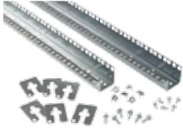
24-in. Rack Angles are available in both square-hole and tapped-hole designs. Tapped Rack Angles are 12 gauge plated steel with 10-32 tapped holes. Square-Hole Rack Angles are 14 gauge plated steel designed to accept metric or English cage nuts. 24-in. Rack Angles fit directly into 700- or 800-mm wide frames using Frame Reducing Brackets.
