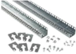
19-in. U-Shaped Rack Angles are available in square-hole and tapped-hole designs. Tapped Rack Angles are 12 gauge plated steel with 10-32 tapped holes. Square-Hole Rack Angles are 14 gauge plated steel designed to accept metric or English cage nuts. 19-in. Rack Angles are fixed directly into a 600-mm wide enclosure frame. To mount 19-in. Rack Angles in 700- or 800-mm wide frames, use Frame Reducing Brackets.
