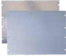
Rack Panels are available in aluminum and painted steel. Aluminum Rack Panels are .125-in.-thick 5052-H32 alloy. Steel Rack Panels are 12 gauge steel and finished in RAL 7035 textured light-gray polyester powder paint. All panels are flat with oblong holes positioned at EIA standard spacing. Mounting hardware is sold separately.
