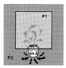
Temperature-related pressure differences between the inside of the enclosure (P1) and the surrounding atmosphere (P2) are balanced by the breather. The amount of condensation forming in the enclosure is thus kept to a minimum.
