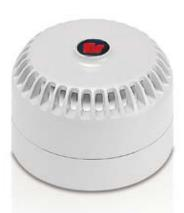
Model LP4 low profile, electronic piezo sounder is a compact multi-tone sounder ideal for OEM and general alarm applications. The low voltage LP4 provides users with the choice of 32 different tones, selectable during installation. Each electrical connection has two terminals for looping in and out, eliminating the need for a separate terminal block, making installation easier. A second tone is available if a third wire is installed and connected to the second tone terminals.
