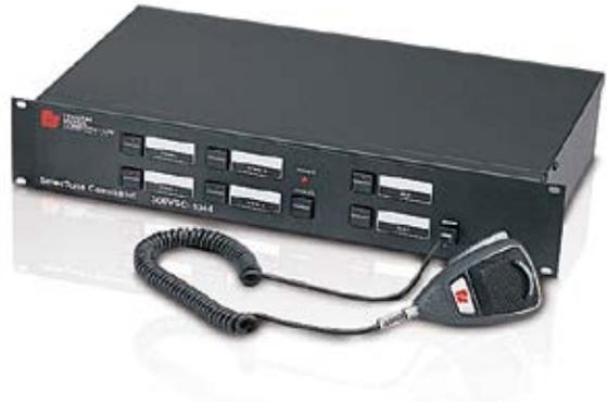
Model 300VSC-1044SB SelecTone® Command Unit generates up to four tones or voice communications in a SelecTone system. The housing can be mounted in any standard 19" equipment rack. Four tones, auxiliary, test and cancel are controlled via an illuminated keypad. Voice transmission is activated by keying the optional desktop or hand-held microphone.
