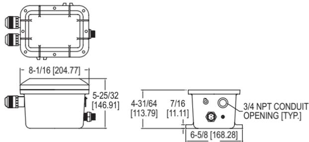
The **SERIES TR-7** Safe-T-Ground provides continuous monitoring of a truck's ground connection throughout loading operations. The TR-7 instantly stops loading operations if a tank truck loses its ground. To safeguard loading operations, the Safe-T-Ground circuit can be wired into your pump control, and to an audible alarm or signal light.
