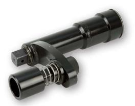
The TrukTorque™ nose extension features a special curved reaction arm designed to handle bolt tightening on the front and rear wheels of trucks and buses. The design easily accommodates wheel trims and deeply recessed wheel bolts.
