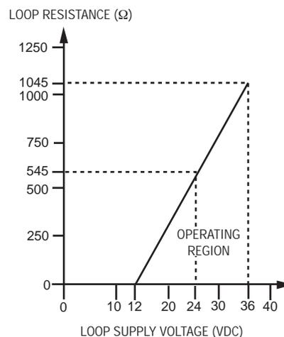
$$V_{\min} = 12V + (.022A \times R_L)$$
