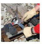
• Used to remove the slag from the crucible area of the mold after making a nVent ERICO Cadweld connection
