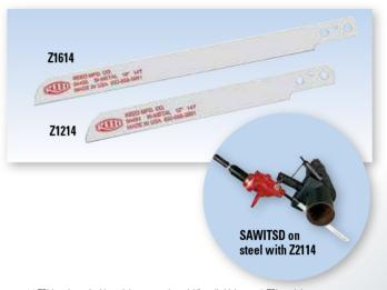
14 TPI (teeth per inch) work best on at least 1/8" wall thickness. 8 TPI work best on walls at least 3/16" thick. Choose 8 teeth per inch for softer materials like plastic.
