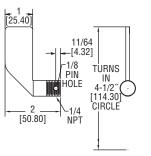
**PDL-4.** 316 SS single vane paddle for heavy weight materials with a minimum bulk density of 70  $lb/ft^3$  (1122 kg/m<sup>3</sup>). Fits through 1-1/4" coupling eliminating the need for a mounting flange.
