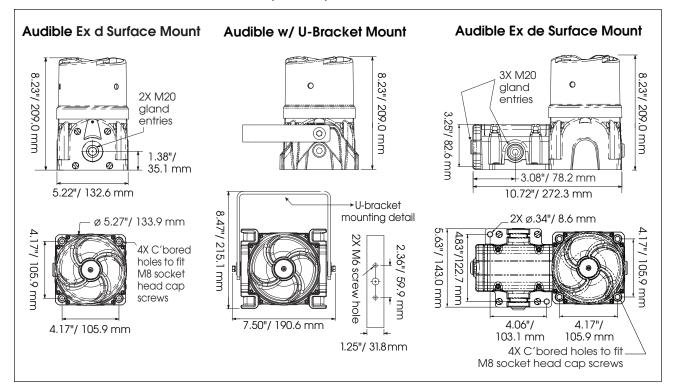
Operating Temperature: -67°F to 158°F -55°C to 70°C Certification Marking: Ex db IIB T5 Gb or Ex db e IIB T5 Gb Ex tb IIIC T100°C Db IP66
